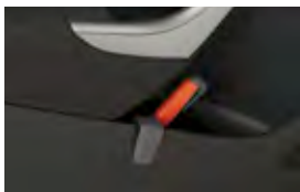
Clamp fastener for car door Quick Click System
